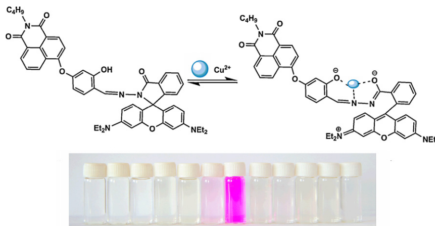
Scheme 2. Binding mode of NRC with \text{Cu}^{2+} . Bottom: photograph of NRC ( 10 \mu\text{M} ) as a selective naked-eye chemosensor for \text{Cu}^{2+} in ethanol–water solution (v/v, 1:9, 50 mM HEPES, pH 7.0), upon addition of 100 \mu\text{M} individual metal ion including \text{Na}^+ , \text{Ag}^+ , \text{Mg}^{2+} , \text{Zn}^{2+} , \text{Pb}^{2+} , \text{Fe}^{3+} , \text{Cu}^{2+} , \text{Mn}^{2+} , \text{Cd}^{2+} , \text{Ni}^{2+} , \text{Co}^{2+} , and \text{Hg}^{2+} (from left to right).
