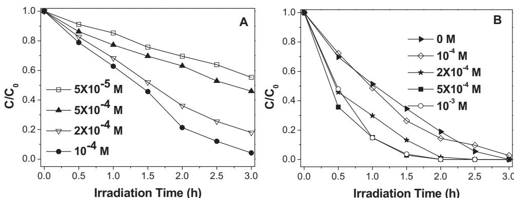
**Fig. 2.** The effects of (A) 2,4,6-TCP initial concentration on Cr(VI) ( $2 \times 10^{-4}$  M) reduction and (B) Cr(VI) initial concentration on 2,4,6-TCP ( $1 \times 10^{-4}$  M) degradation.
