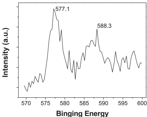
**Fig. 6.** Cr 2p spectrum of chromium on  $\text{g-C}_3\text{N}_4$  after photoreaction.
