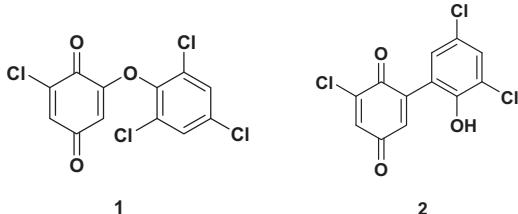
**Fig. 7.** Structures of the identified coupling products in the 2,4,6-TCP/Cr(VI)/ $\text{g-C}_3\text{N}_4$  complex system after 0.5 h photoreaction.
