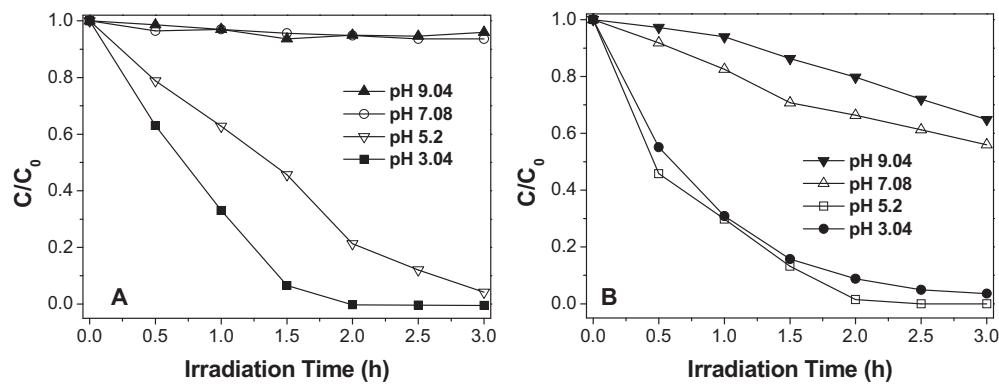
**Fig. 3.** (A) Cr(VI) reduction and (B) 2,4,6-TCP degradation at different pH condition in the 2,4,6-TCP/Cr(VI)/g-C<sub>3</sub>N<sub>4</sub> reaction system.
