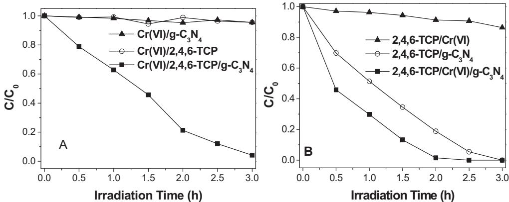
**Fig. 1.** The synergistic effect of Cr(VI) reduction and 2,4,6-TCP degradation over  $\text{g-C}_3\text{N}_4$  under visible light irradiation: (A) Cr(VI) reduction and (B) 2,4,6-TCP degradation.
