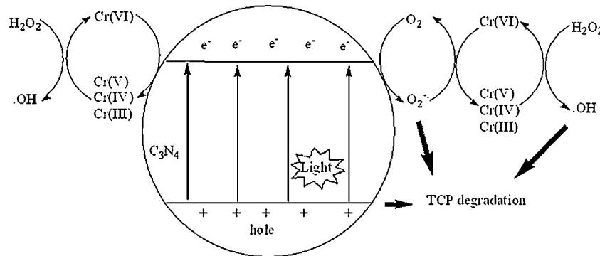
**Fig. 10.** Reaction pathway of Cr(VI) reduction and 2,4,6-TCP degradation over  $\text{g-C}_3\text{N}_4$  under visible light irradiation.
