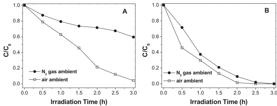
**Fig. 4.** (A) Cr(VI) reduction and (B) 2,4,6-TCP degradation at different ambient in the 2,4,6-TCP/Cr(VI)/g-C<sub>3</sub>N<sub>4</sub> reaction system.
