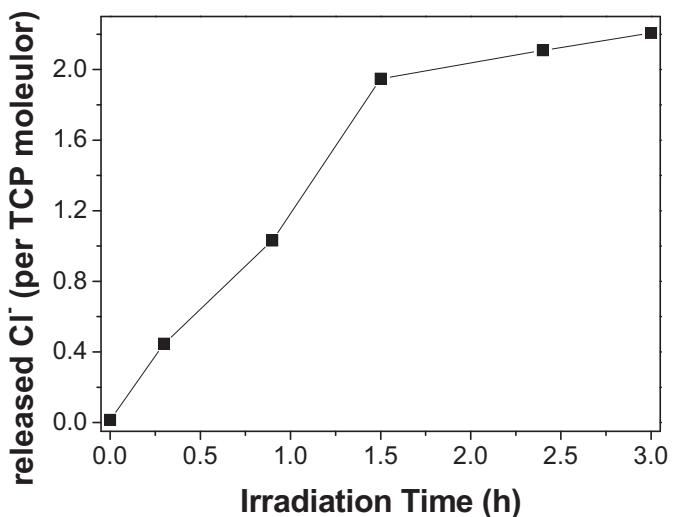
**Fig. 8.** Chloride ions release during 2,4,6-TCP degradation in the 2,4,6-TCP/Cr(VI)/ $\text{g-C}_3\text{N}_4$  system under visible light irradiation.
