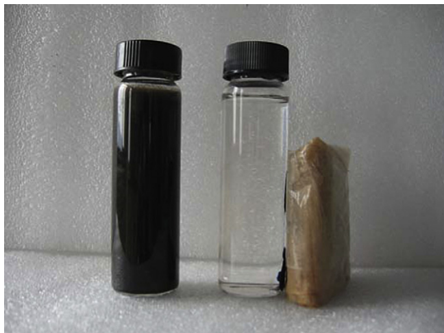
Fig. 3. Magnetic separation of well-dispersed \text{MnFe}_2\text{O}_4 /activated carbon composite from solution under external magnetic field.
