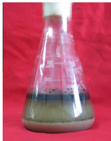
Fig. 1. The three phases separate of sludge after treated by the culture medium of BZ-6.
