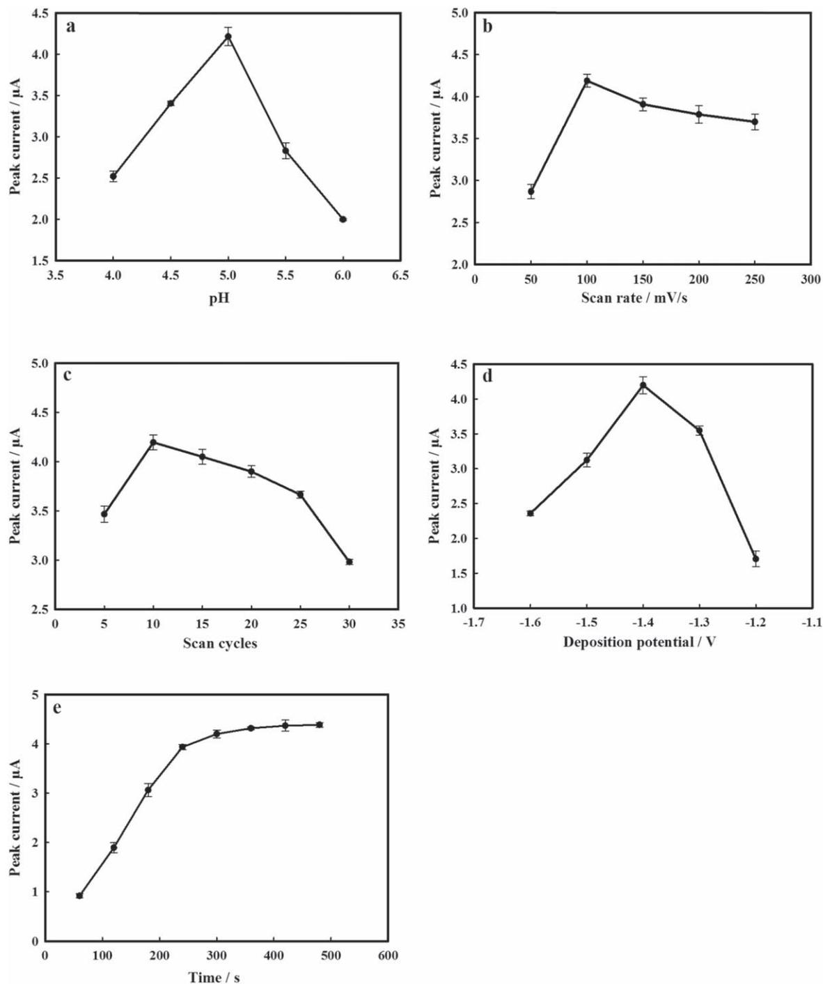
**Figure 6.** Effects of the pH values (a) of acetate buffer solution, scan rate (b) and the scan cycles (c) of 0.2 mM PSS, deposition potential (d) and the deposition time (e) on the DPV peak current for 230 nM Zn(II) in 0.1 M acetate buffer solution at the PSS/W-rGO/GCE.  $n = 3$ .
