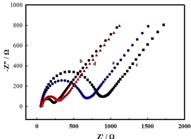
Figure 4. Nyquist plots of bare GCE (a), W-rGO/GCE (b), PSS/GCE (c), and PSS/W-rGO/GCE (d) in  $0.1 \text{ M KCl}$  solutions containing  $5 \text{ mM Fe(CN)}_6^{3-/4-}$ .
