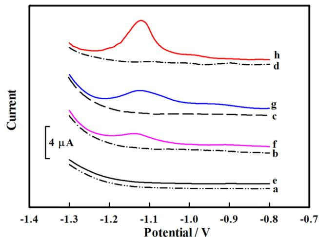
Figure 5. DPV response curves in  $0.1 \text{ M}$  acetate buffer (pH  $5.0$ ) without (a)–(d) and with (e)–(h)  $230 \text{ nM Zn(II)}$  at bare GCE (a), (e), W-rGO/GCE (b), (f), PSS/GCE (c), (g), and PSS/W-rGO/GCE (d), (h). Parameters: amplitude of  $0.05 \text{ V}$ , pulse width of  $0.2 \text{ s}$ , pulse period of  $0.5 \text{ s}$ , and an equilibrium time period of  $2 \text{ s}$ .
