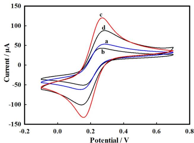
Figure 3. Cyclic voltammograms of  $5 \text{ mM Fe(CN)}_6^{3-/4-}$  in  $0.1 \text{ M KCl}$  solution at bare GCE (a), PSS/GCE (b), W-rGO/GCE (c), and PSS/W-rGO/GCE (d).
