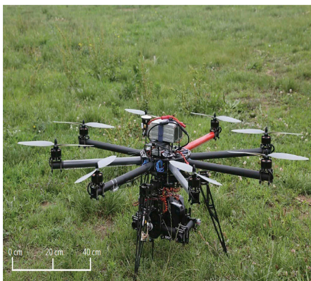
Figure 2. The rotary-wing (eight rotors) UAVs (ZH3-600, Qingdao, China).
