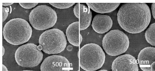
**Fig. 1** SEM images of the obtained (a) MIP and (b) NIP beads.
