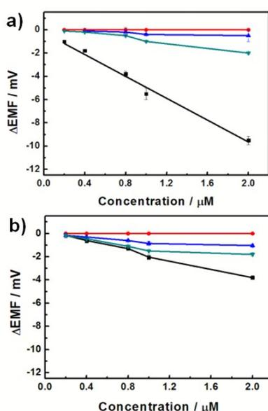
**Fig. 5** Potentiometric selectivity of the MIP (a) and NIP (b) membrane-based sensors towards neutral phenols: (■), BPS; (▼), 2-phenylpheno; (▲), 4,4'-dihydroxybiphenyl; (●), phenol. Other conditions are as given in Fig. 3. Error bars represent one standard deviation for three measurements.
