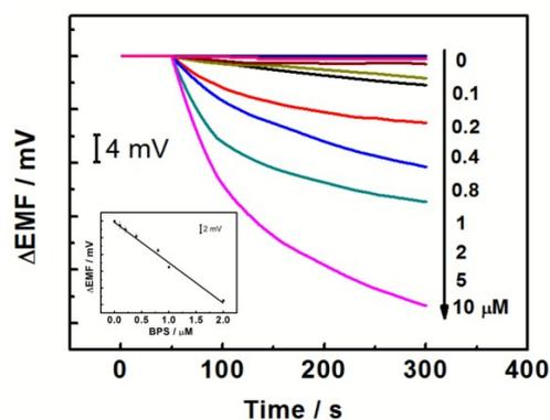
**Fig. 4** Typical potential responses of the solid-contact electrode based on MIP to neutral BPS in the concentration range of 0.1 to 10  $\mu\text{M}$ . The inset shows the calibration curve for neutral BPS detection. Other conditions are as given in Fig. 3. Error bars represent one standard deviation for three measurements.
